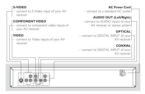
Caution: Do not touch the inner pins of the jacks on the rear panel. Electrostatic discharge may cause permanent damage to the unit.
